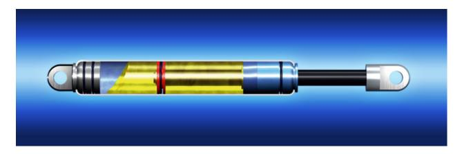
MC-damper standard This specification with damping over the complete stroke contains only oil. Due to the construction, there will be a small slip when the piston rod is pulled out. The push-in and push-out speed – i. e. the effective slowing down (motion control) of the movement of a mass – can be influenced considerably by the use of different nozzles as well as by different oil viscosities.
