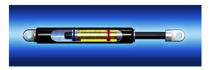
MC-damper without slip This easylift damping variety allows a controlled damping in both directions, without slip effect. Here, the piston moves completely in a fixed oil chamber.
